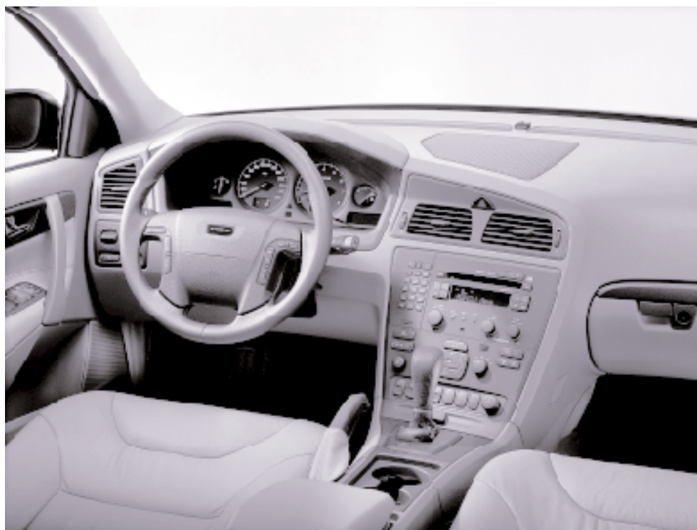
Volvo V70 CYCOLOY IP carrier made of CYCOLOY resin
